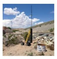
Alert 2 Flood Warning System. This system includes standard weather stations (rain gauge, measuring devices, and stream gauge) and an advanced communication technology to transmit rainfall and other data to a central location. Additionally, the plan will provide a high-level overview for flood risk regions within the City and DAC, propose site locations for future flood warning systems, and set budgets for maintenance, operations and expansion.
