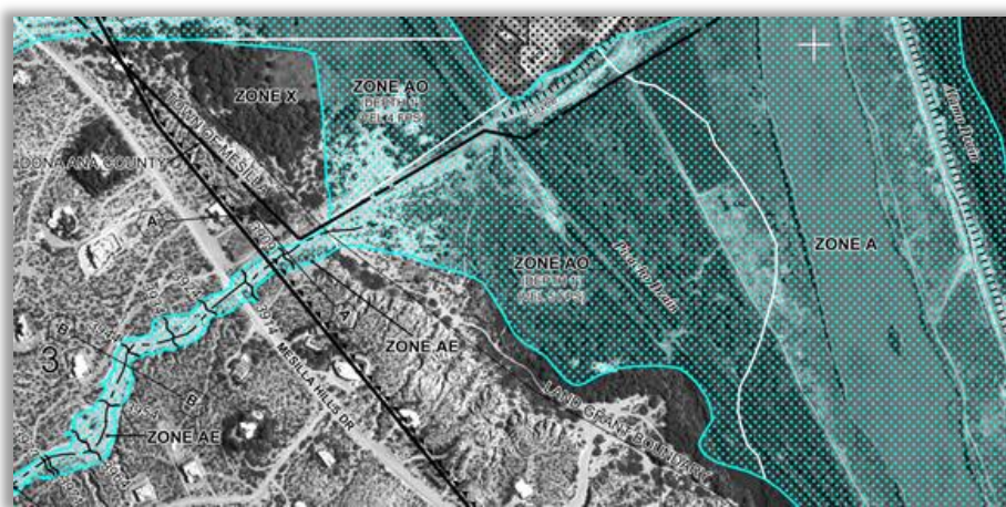
Figure 5-8. Example of unnumbered A Zone on a FIRM. The detailed study is designated by the "AE" and "AO" Zone
